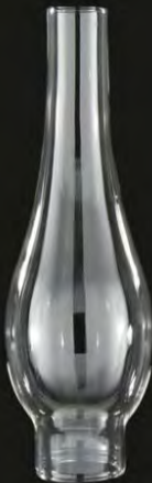
57910 - 1 5/8" fitter, 8 1/2" ht. with 2 3/4" bulge, clear chimney. Fits Gem Arctic and #0 Hornet burner
