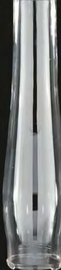
57951 - 2 5/8" fitter, 13" ht. with 2 7/8" bulge, clear "Twist-Lock" chimney* to fit Aladdin® brand burner models 7-12, A,B,C, 21, 21C, & 23, and B & P replacement burners #30241 thru #30249
