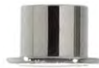
Ferrules with flange , 3/4" inside dia., outside dia. slips 7/8" hole. Tap 1/8F 21081C - Chrome Plated Finish 21081 - Brass Plated Finish
