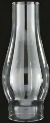
57930 - 2 5/8" fitter, 8 1/2" ht. with 3 5/8" bulge, clear chimney. Fits Rayo & Central Draft burners, reg. bulge chimney
